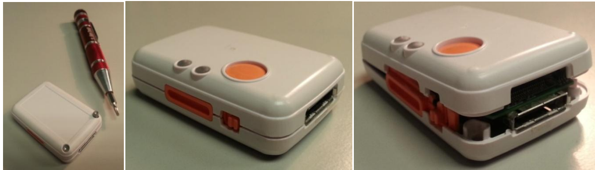
Figure 9-3 Opening the enclosure
