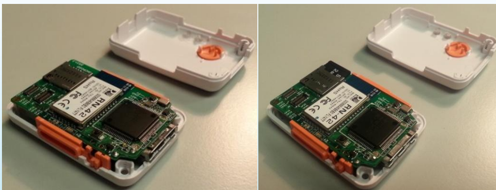
Figure 9-7 Installed circuit board and SD card insertion
