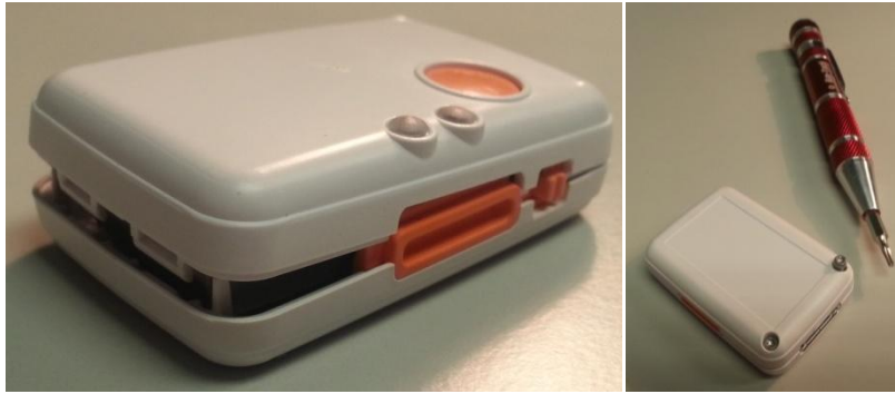
Figure 9-8 Closing the enclosure and inserting screws
