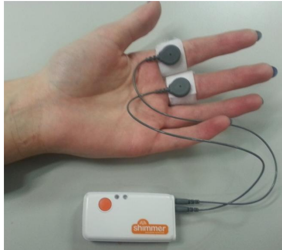
Figure 3-1: Example electrode positioning for GSR
