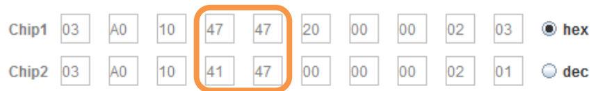
Figure 3-5: A zoomed in view of the MUX bytes as they appear in Consensus. Note that within each of these bytes, Bits [3-0] control the MUX settings, Bits [6-4] control each channel's gain ( i.e. , Gain = 4 in this case) and Bit [7] is fixed at 0.
